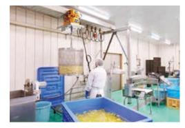
are required to maintain rigorous hygiene control as well as safety control of the equipment and machines they use. To keep foreign matter out, the hoist comes with a dustpan.
