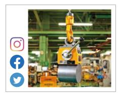
Equipped with permanent magnets, a single unit is enough for safe, reliable handling of both flat and round steel.
