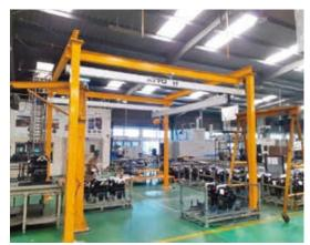
Kito India recently wrote its first order for the PRO light Crane System for a local joint venture related to a Japanese heavy-industrial-machine maker. It is used to transport the diesel engines produced there. The firm previously used a steel crane, and our emphasis on the lightness and easy operability of the aluminum crane led to the order. With the recent beginning of construction on several power stations in India, many Kito products are at work there.
